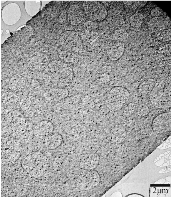
Fig. 10. Longitudinal section of a BN fibre.
